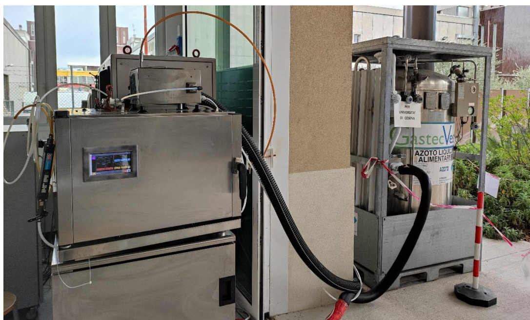
Figure 1. Prototype of salmon cryo-smoker and liquid nitrogen tank connected to the machine.
