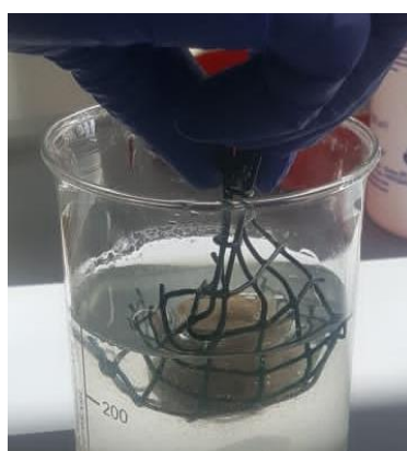
Figure 4. Application of chitosan coating by immersion (dipping) in 1% (w/v) solution
