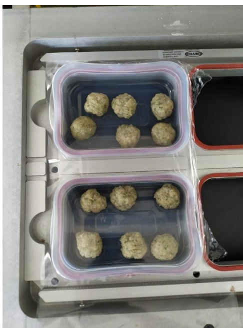
Figure 6. Fish-balls packed in 20% CO 2 -80% N 2 using a vacuum-compensated packaging machine
